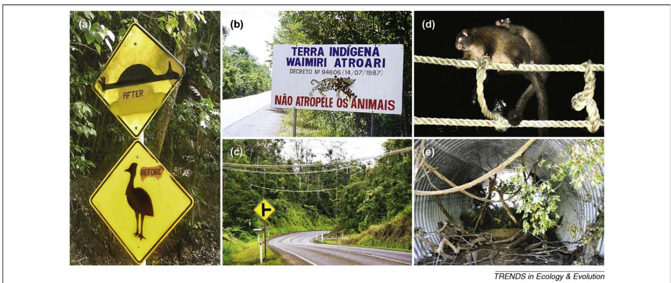
Figure 5. Efforts to mitigate road impacts: warning signs for motorists in tropical Queensland (a) and Brazil (b); artificial walkways for arboreal wildlife in Queensland (c), which enable road crossing by sensitive species such as the lemuroid ringtail possum ( Hemibelideus lemuroides ) (d); and wildlife-friendly culverts under roads in Queensland (e). Reproduced with permission from W. Laurance (a, b), M. Goossem (c, e) and J. Cooper (d).
